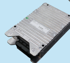
VCU system is comprised of two parts which may be mounted separately near each other. In this application, they are mounted on a swing panel, one on each side.
